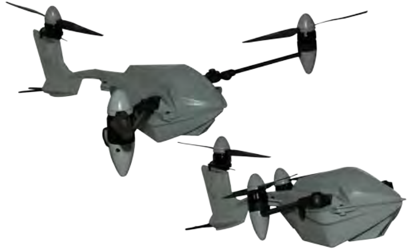
“Bullray” Amphibious Tri-copter UAS (Fiber reinforced FDM) - Sketch to Flying Prototype in 3 Months
