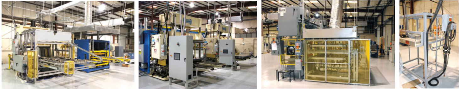
Custom, Fully Automated Composite Shuttle, Thermoplastic Heater and Press Systems up to 600A, 480V, 3/PHASE.
